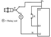
Use relay coil Voltage of the same Voltage using for Proximity sensor. [Relay coil current should not exceed the maximum current Specified by Proximity sensor.]
