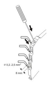
The module has been designed for spring-type terminal electrical connections.
