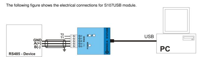
By inserting an external bridge between T1 and T2 terminals, the terminator of the RS485 line is inserted. In case of long connections or noisy environments, it is advisable to use screened cables for the RS485 line.
