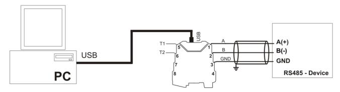
By inserting an external bridge between T1 and T2 terminals, the terminator of the RS485 line is inserted. In case of long connections or noisy environments, it is advisable to use screened cables for the RS485 line.
