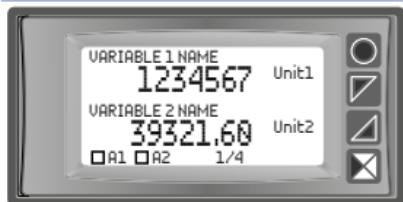
Shows the value of the first two variables enabled with relative description, unit of measurement and status of the alarm relays. The figure represents the display of "2 val. per page" setting in "Display -> View" parameter.
