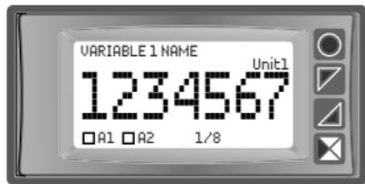
Shows the value of the first variable enabled with relative description, unit of measurement and the status of the alarm relays. The figure represents the display of "1 val. per page" setting in "Display -> View" parameter. The 1/8 text at the bottom indicates that the first of 8 pages used to represent enabled variables is being displayed.
