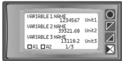
Shows the value of the first three variables enabled with relative description, unit of measurement and status of the alarm relays. The figure represents the display of "3 val. per page" setting in "Display -> View" parameter.
