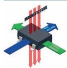
When a magnetic field is applied perpenducularly to a conductor, a transverse voltage is generated to the direction of current flow. Hall effect transducers are used as alternative to the shunt when dealing with high voltages and high galvanic isolations.
