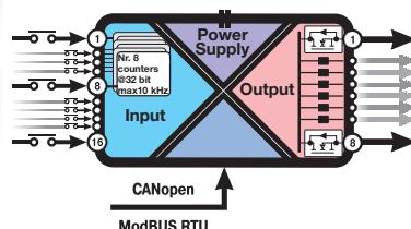
ZC-16DI-8DO is an 16 CH input / 8 CH output mixed module. The inputs have 32-bit counters / 10 kHz max frequency, mosfet Outputs with shared negative pole. The communication protocols are CANopen or ModBUS RTU (protocol selectable through dip-switch). A 3-way galvanic isolation among Power supply // input // RS485 circuits assures the integrity of your datas
