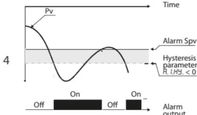
Absolute alarm with controller in cooling functioning (Par.7 *Rct.L.* selected *Cool*) and hysteresis value less than "0" (Par.29 *R.I.HY. < 0*).\*
