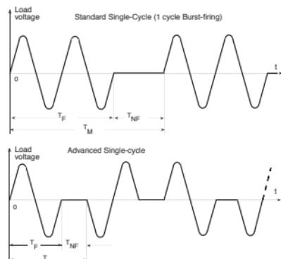
For a percentage less than 66%, SSR output firing takes place as in the "Burst fire" mode (see b5E.F.)
