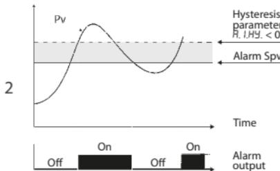
Absolute alarm with controller in heating functioning (Par.7 *Rct.L.* selected *HEAT*) and hysteresis value less than "0" (Par.29 *R.I.HY. < 0*).\*
