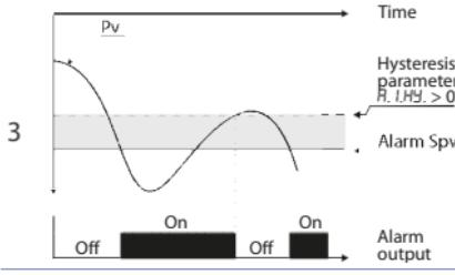
Absolute alarm with controller in cooling functioning (Par.7 *Rct.L.* selected *Cool*) and hysteresis greater than "0" (Par.29 *R.I.HY. > 0*).\*
