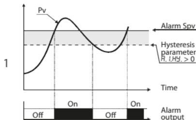
Absolute alarm with controller in heating functioning (Par. 7 *Rct.L.* selected *HEAT*) and hysteresis value greater than "0" (Par.29 *R.I.HY. > 0*).\*
