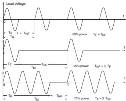
**At 50% power, the modulation time is 40ms:**
