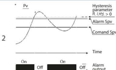
Lower deviation alarm value of alarm setpoint less than "0" and hysteresis value greater than "0" (Par.29 R.I.HY. > 0).\*\*
