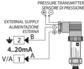
For linear signals 0/4..20 mA with external power supply for sensor.
