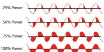
Using a no zero-crossing SSR, the ATR227 synchronizes with the power supply voltage (necessarily AC) and determines when to activate the output to create the right choking.
