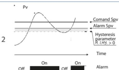
Upper deviation alarm value of alarm setpoint less than "0" and hysteresis value greater than "0" (Par.29 R.I.HY. > 0).\*\*
