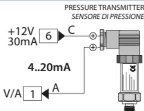
For linear signals 0/4..20 mA with two-wires sensors.
