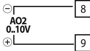
**Pins 8-9:** linear output in Volt configurable using parameters as retransmission of process or alarm setpoints (vedi par. 119-123).
