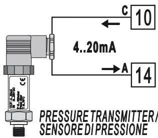
For linear signals 0/4..20 mA with **two-wire sensor**.
