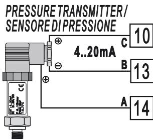
For linear signals 0/4..20 mA with **three-wire sensor**.
