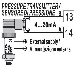
For linear signals 0/4..20 mA with **external power of sensor**.
