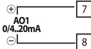
**Pins 7-8:** linear output in mA configurable using parameters as retransmission of process or alarm setpoints (see par. 112-116).
