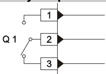
Capacity 5A/250V~ for resistive loads
