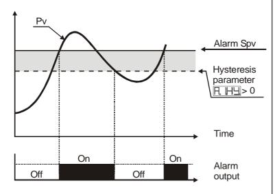
Absolute alarm with controller in heating functioning (Par.11 FLEE selected HEFE) and hysteresis value greater than "0" (Par.28 F. HY) > 0).
