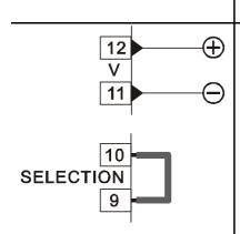
Linear output in <u>Volt</u> configurable using parameters as command (Parameter ) or retransmission of process or setpoint (Parameter ).
