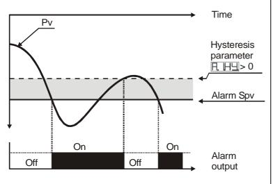
Absolute alarm with controller in cooling functioning (Par.11 FLL) selected LDD and hysteresis value greater than "0" (Par.28 FL HH) > 0).
