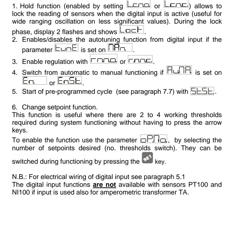
Digital input is programmable for several functions which are useful to simplify controller operability. Select the desired function on parameter
