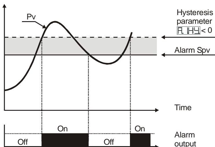
Absolute alarm with controller in heating functioning
