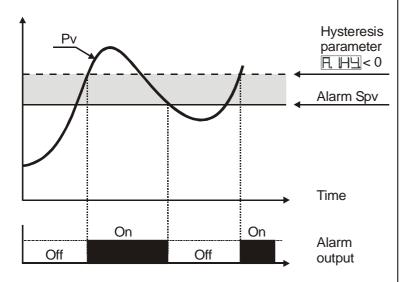
Absolute alarm with controller in heating functioning (Par.11 FLEE selected HERE) and hysteresis value less than "0" (Par.28 FLEE < 0).
