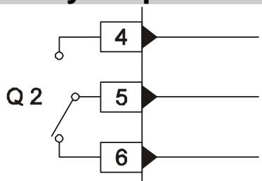
Capacity 5A/250V~ for resistive loads
