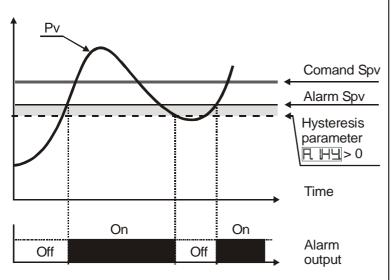
Upper deviation alarm <u>value of</u> <u>alarm setpoint less than "0"</u> and <u>hysteresis value greater</u> <u>than "0"</u> (Par.28 []. [H] > 0).
