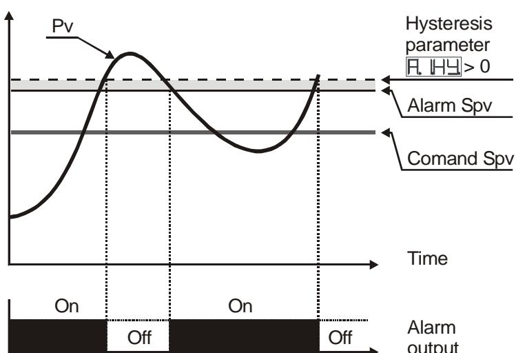
Lower deviation alarm value of alarm setpoint less than “0” and hysteresis value greater than “0” (Par.28  $R_{IH}$  > 0).
