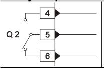
Capacity 5A/250V~ for resistive loads
