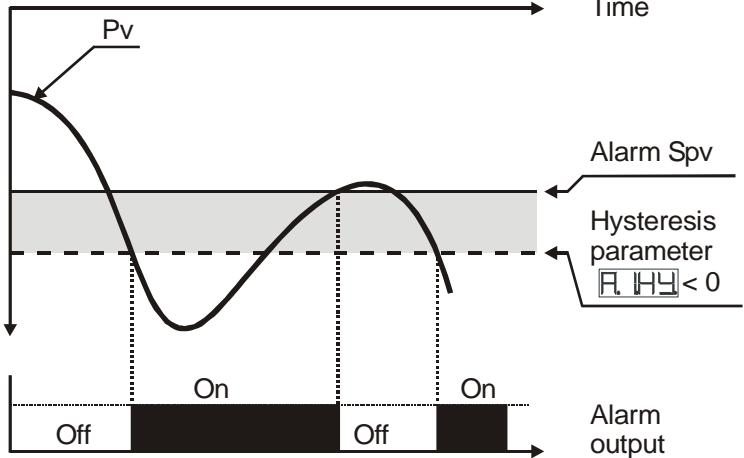
Absolute alarm with controller in cooling functioning
