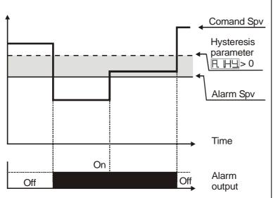
Absolute alarm refers to the command set, with the controller in heating functioning
