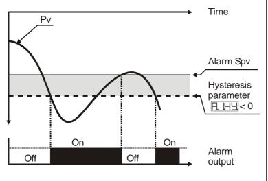
Absolute alarm with controller in cooling functioning (Par.11 FLE selected and hysteresis value less than "0" (Par.28 F. HH < 0).
