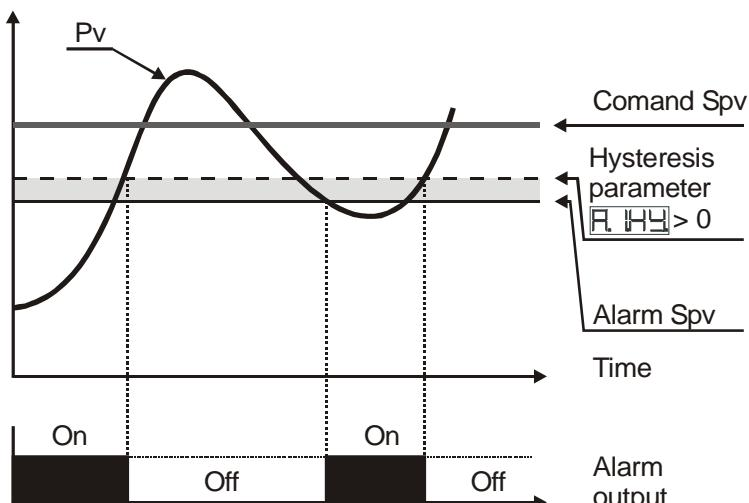
Lower deviation alarm value of alarm setpoint greater than “0” and hysteresis value greater than “0” (Par.28  $R_{IH}$  > 0).
