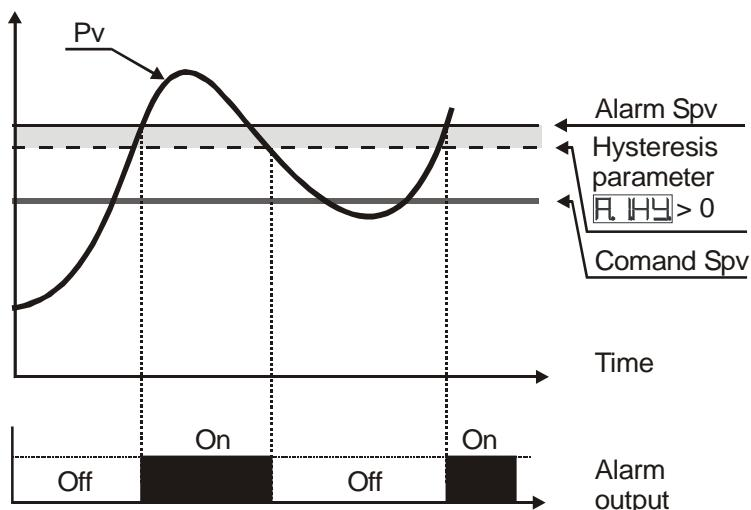
Upper deviation alarm value of alarm setpoint greater than "0" and hysteresis value greater than "0" (Par.28  $R_{IH4} > 0$ ).
