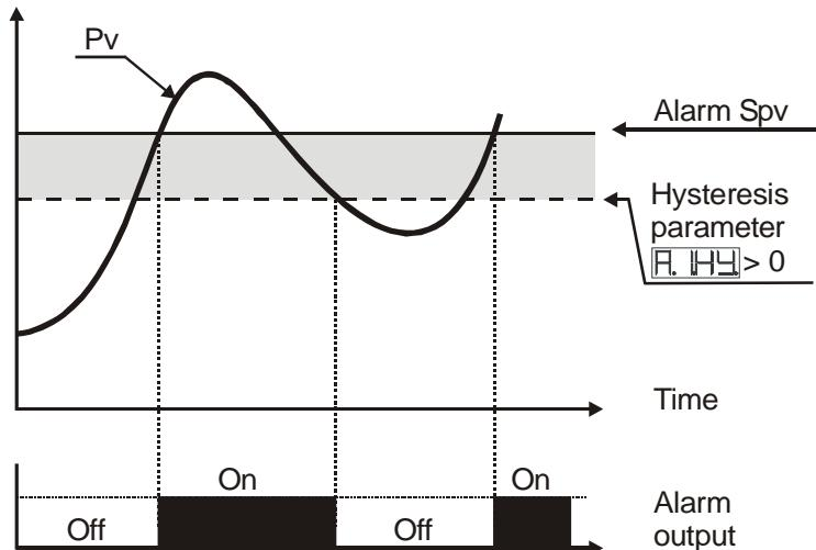
Absolute alarm with controller in heating functioning
