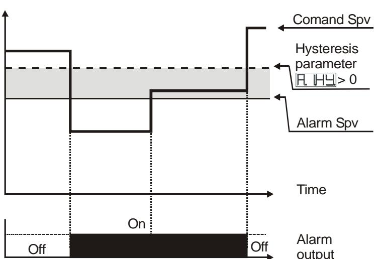
Absolute alarm refers to the command set, with the controller in heating functioning
