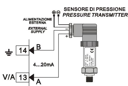
Linear signals 0/4....20mA with **external power of sensor**
