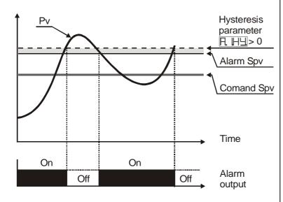
Lower deviation alarm <u>value of</u> <u>alarm setpoint less than "0"</u> and <u>hysteresis value greater</u> <u>than "0"</u> (Par.28 日 日 ).
