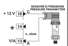
Linear signals 0/4....20mA with **two-wire** sensor
