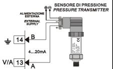
Linear signals 0/4....20mA with **external power of sensor**
