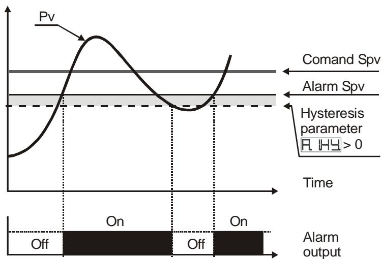
Upper deviation alarm value of alarm setpoint less than "0" and hysteresis value greater than "0" (Par.28  $R_{IH4} > 0$ ).
