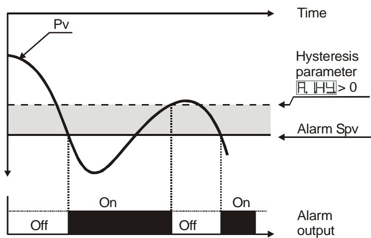
Absolute alarm with controller in cooling functioning
