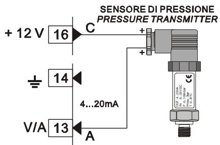
Linear signals 0/4....20mA with **two-wire sensor**
